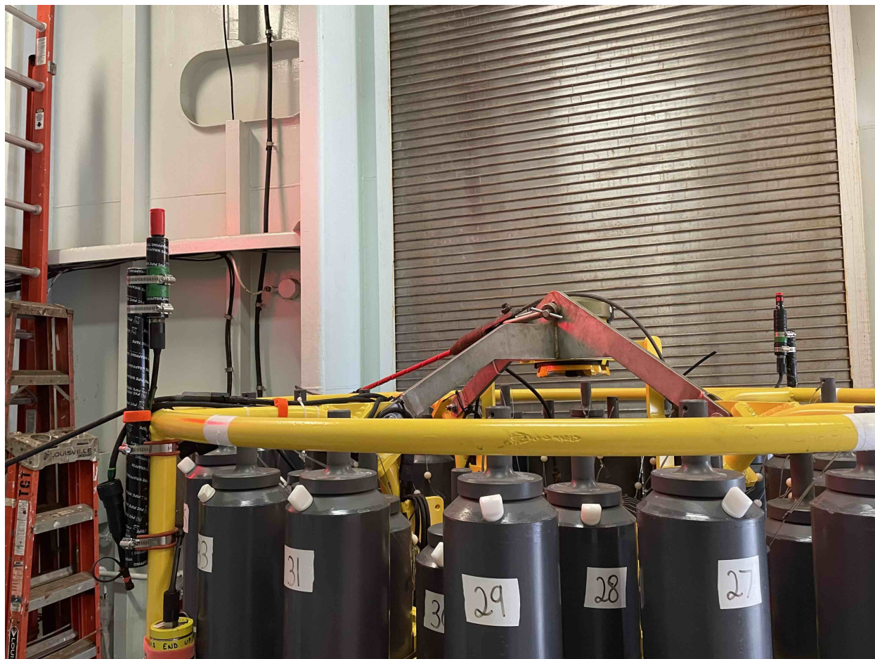
Fig. 1: Upward-looking chipod sensors attached to the rosette.
