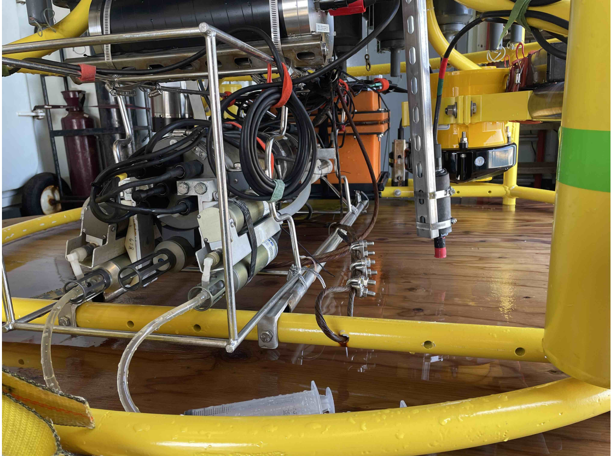
Fig. 5: Package setup from southwest, with CTD in foreground and downlooking chipod to the right.
