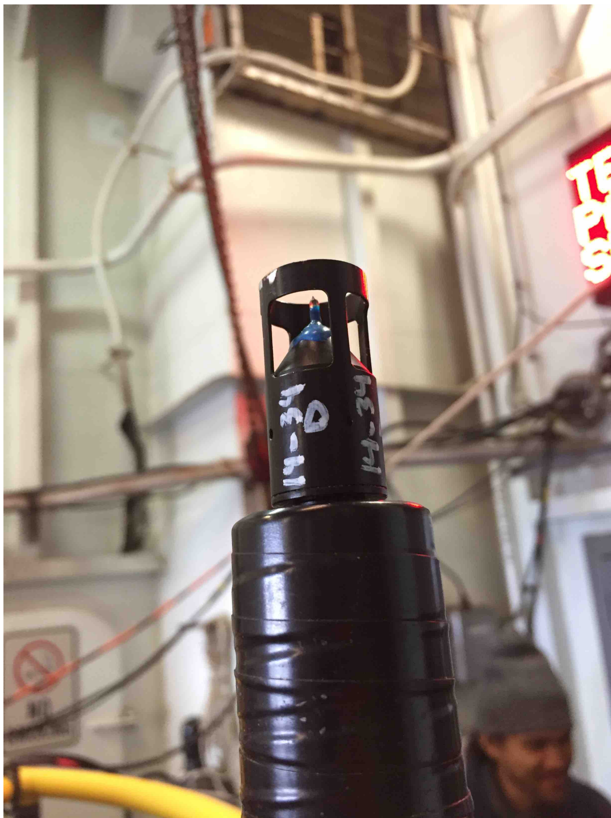
Fig. 3: Highly sensitive temperature probe, which is sampled at 100Hz.
