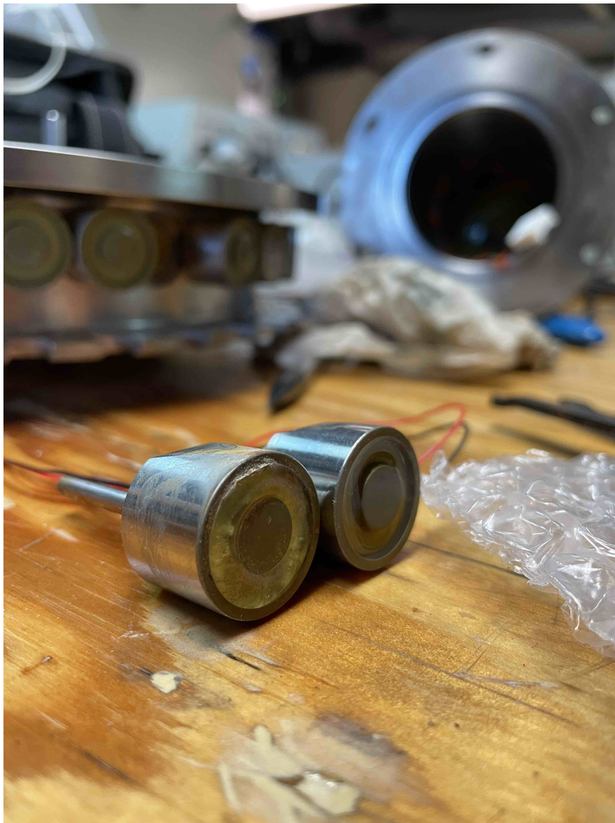
Fig. 9: Bad solenoid (left), cloudy and raised edge from corrosion.
